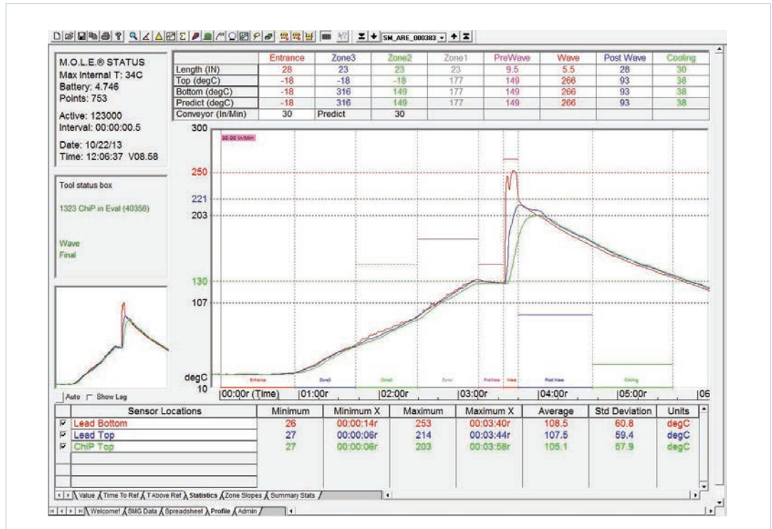
Figure 1 Preferred Soldering Process Profile
